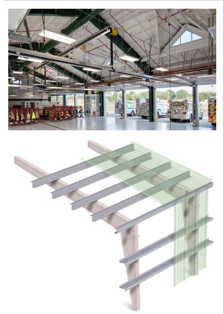
Illustration of secondary structural steel framing (girts/purlins) supporting the metal roof panel (standing seam or through fastened) and metal wall panel (through fastened) cladding. The girts and purlins are attached to the primary structural steel framing.
